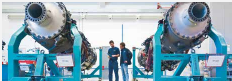
MTU is responsible for the final assembly and production acceptance testing of all TP400-D6 production engines.
