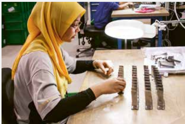
Close examination: visual inspection of engine blades
