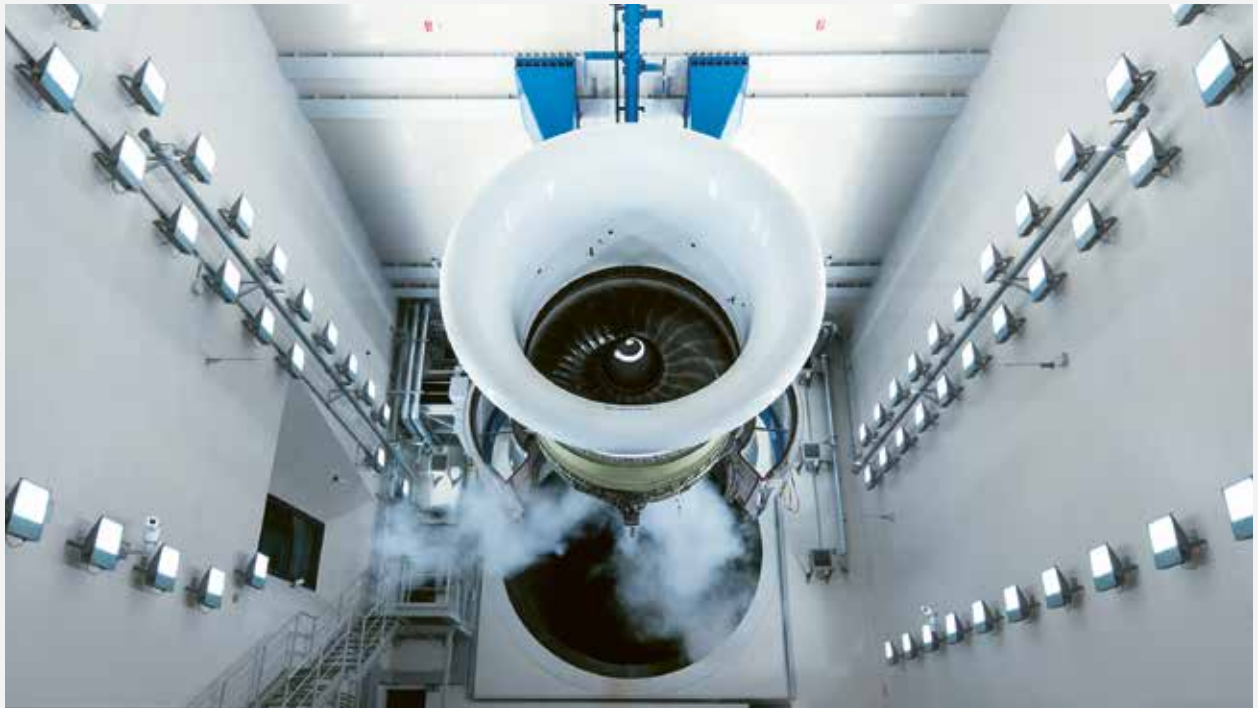
A freshly overhauled GE90 Growth engine must undergo an acceptance test run—in line with the scope of the shop visit. There are two test cells at the Hannover location: with a thrust range up to 100,000 pounds and 150,000 pounds, respectively.
